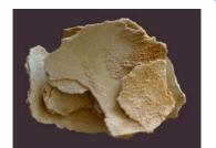
**Calcite**, a form of calcium carbonate, is what we call limescale or scale. When calcium carbonate precipitates as calcite it forms a hard deposit that causes numerous problems adhering to any receptive surface requiring acid or a significant mechanical effort to remove.
